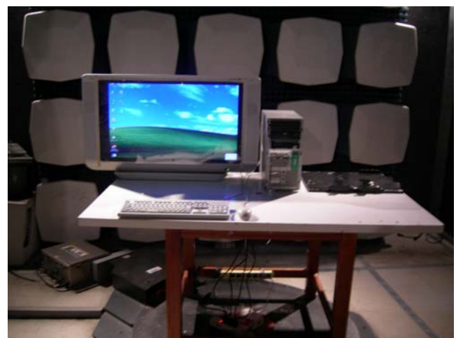
Fig. 5 Setup test device in EMI chamber
